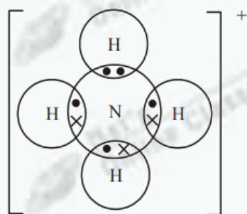
'Dot-and-cross' diagram to show four shared pairs of electrons one of which is a dative covalent bond (which must consist of the same symbols) ✓
