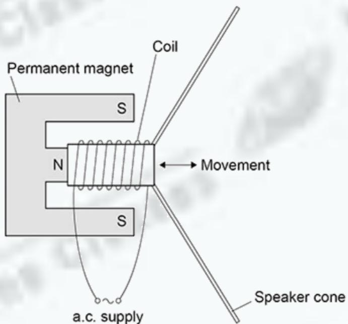
(a) What is the name of the effect used by the moving-coil loudspeaker to produce sound waves?
