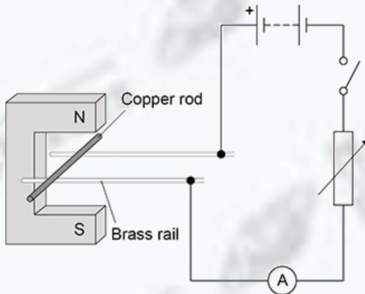
(a) The teacher closes the switch and the copper rod accelerates.
